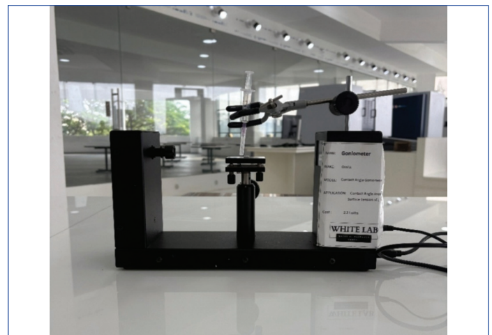
[Table/Fig-9]: Ossila goniometer for measuring the contact angle.
